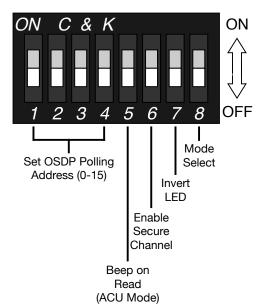
**DIP Switches 1-4:** Set the OSDP Polling Address in PD mode. Set the OSDP Address to be polled by the OSM unit in ACU mode. See the DIP Switch Address Table to the right.
